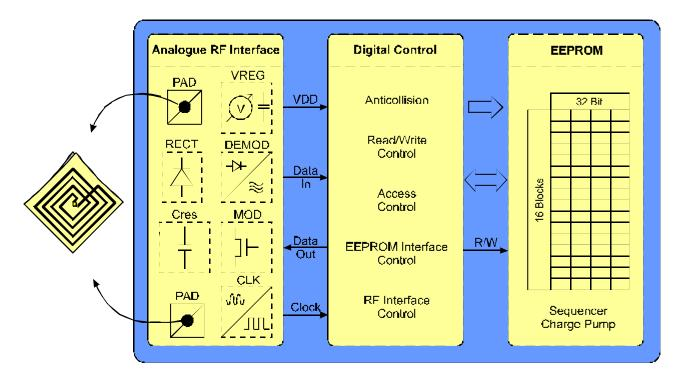
The label requires no internal power supply. Its contactless interface generates the power supply and the system clock via the resonant circuitry by inductive coupling to the reader. The interface also demodulates data that is transmitted from the reader to the I•CODE Label and modulates the electromagnetic field for data transmission from the I•CODE Label to the reader.
